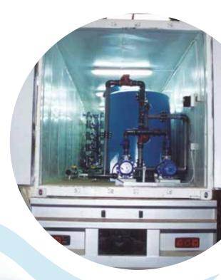
Oil/Water Separations systems have been designed to separate large amounts of oil which has been mixed in with water. Separators have been designed using Stokes Law. Oil/water separators are gravity feed systems, which allows the oil to rise to the top of the water surface then skimmed off and collected in a container. The water is then allowed to pass for further processing.
